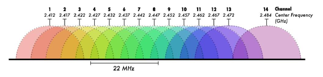
WiFi devices must use the same channel in order to communicate with each other. They send and receive on the same channel, so only one device
