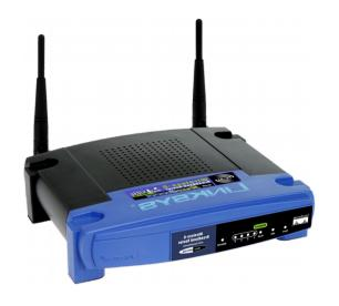
**Master mode** (also called AP or infrastructure mode) is used to provide an infrastructure with an access point connecting different clients. The access point creates a network with a specified name (called the **SSID**) and channel, and offers network services on it.
